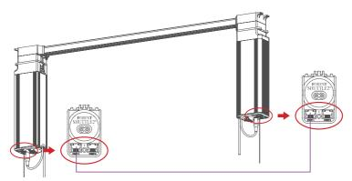
In this master - slave function, two Shuttle M motors are used on one track.
