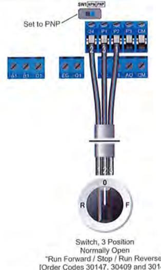
A wiring diagram is shown in the illustration opposite. Ensure that the switch marked "SW1" is set to PNP as shown.
