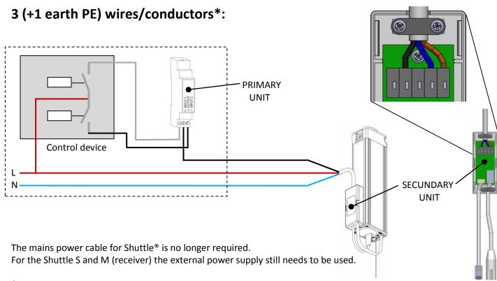
\* The motor must be installed by an installer who is qualified in motorized systems. Installation must be done according to local regulations. Make sure to turn off mains power when installing the units. Earth wire (yellow/green) can never be used as replacement for Live, Neutral or control wire. To ensure safety, the primary unit needs to be mounted in a distribution box, like this:
