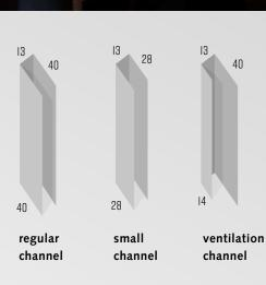
**Please note:** With larger surfaces from approx. 2m<sup>2</sup>, the film may be pushed out of the channels by the heat trapped between the glass and the film (generally in case of narrow and tall systems), which is when it is advisable to use ventilation channels (see illustration)
